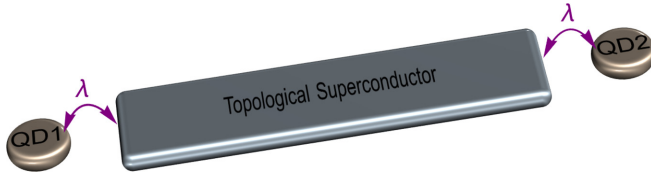
FIG. 1. The schematic of the investigated setup with symmetric coupling \lambda between the quantum dots (QDs) and topological superconducting nanowire, with Majorana modes located at its ends.
