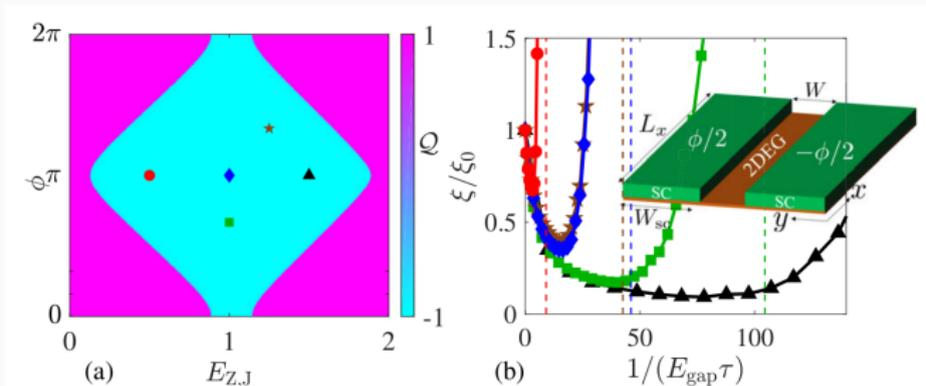
FIG. 1. (a) Phase diagram of the planar Josephson junction Eq. (1) in the clean limit. In the topological phase ( $Q = -1$ ), the system supports zero-energy MBSs at each end of the junction. (b) The Majorana localization length  $\xi$  versus the disorder-induced inverse mean free time  $\tau^{-1}$  for different points inside the topological phase [see markers in (a)].
