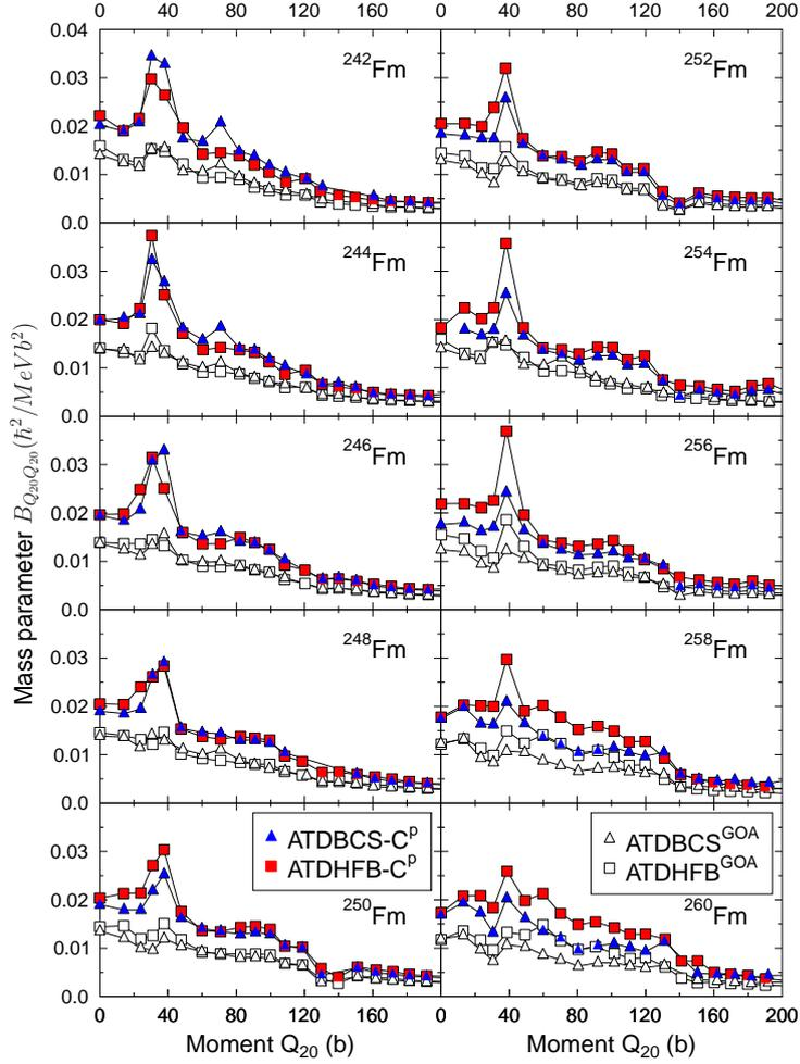
Fig. 2. (Color online) Cranking mass parameter  $B_{Q_{20}Q_{20}}$  (in units  $\hbar^2/\text{MeV b}^2$ ) for Fermium isotopes vs. mass quadrupole moment  $Q_{20}$ . Both GOA (open symbols) and cranking (filled symbols) mass are shown for two types of calculations: HF+BCS (triangles) and HF+FB (squares). In all considered cases the SkM\* force was used.
