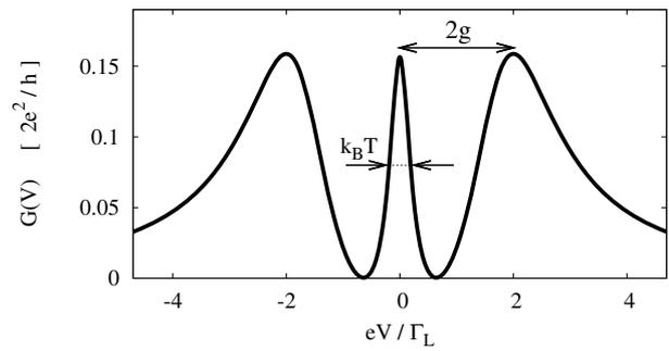
**Figure 2** The differential conductance  $G(V)$  as a function of bias voltage  $V$  for the symmetric case with  $T = 0.2g$  and  $g = \Gamma_L$ . Width of the central (superradiance) peak is proportional to temperature whereas the zero bias value  $G(0)$  still remains constant (temperature-independent) [6].
