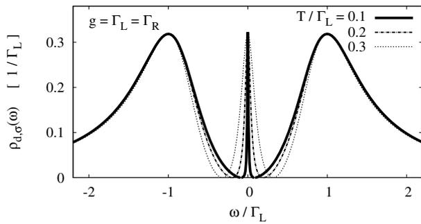
**Figure 1** Spectral function of the molecular quantum dot for the equilibrium situation ( $V = 0$ ) in the symmetric case  $E_{\text{pair}} = 0$ ,  $E_d = 0$  for several temperatures. We used  $g = \Gamma_\beta$  assuming the wide-band limit  $\Gamma_\beta = 0.001D$ , where  $D$  denotes the conduction electron bandwidth.
