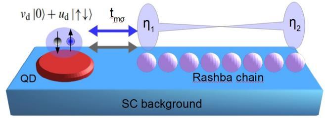
**Figure 1.** Schematic view of the correlated QD side-coupled to the Rashba nanowire and both deposited on SC substrate, where topological SC nanowire hosts two Majorana end-modes  $\eta_1$  and  $\eta_2$ .
