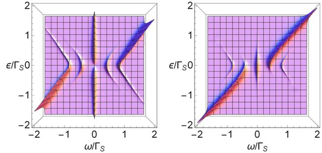
**Figure 2.** Density of states for spin  $\uparrow$  (left) and  $\downarrow$  (right) electrons obtained for  $t_{m\uparrow} = 0.6\Gamma_S$ ,  $t_{m\downarrow} = 0$  in absence of correlations ( $U = 0$ ).
