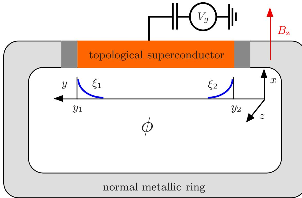
**Majorana-type fermions in hybrid normal–superconducting rings**
