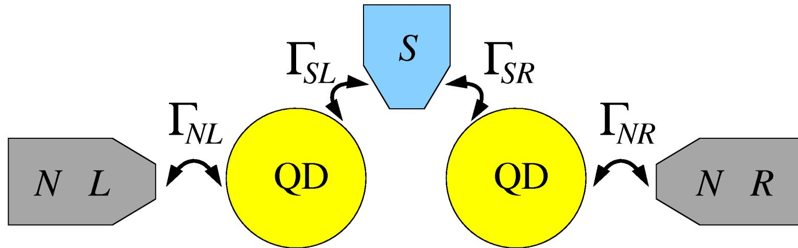
Cooper pairs are depaired by the quantum dots (*quantum forks*).
