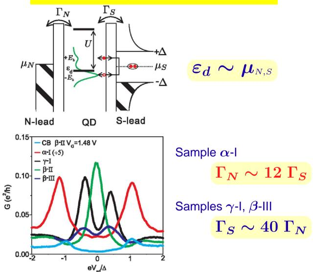
"We attribute the subgap peaks to resonant Andreev transport ... through electron-hole mixing of the QD energy level."
