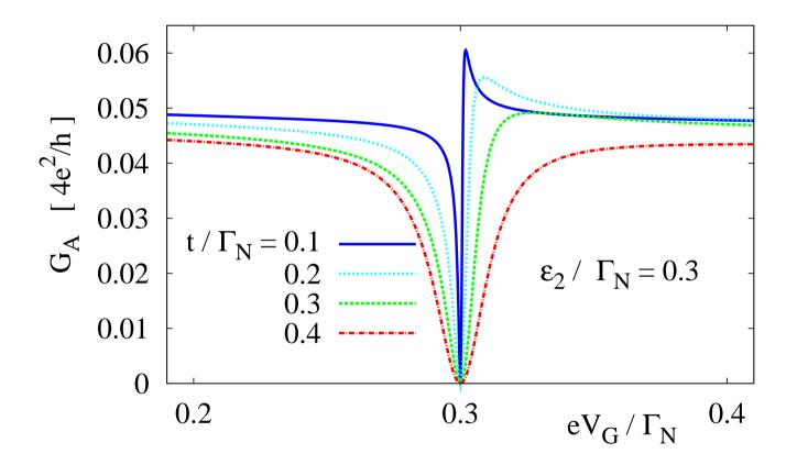
The gate-voltage dependence of  $G_A$  obtained for U=0
