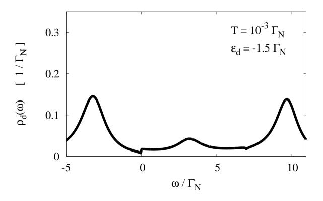
**Superconductivity supresses the Kondo resonance**
