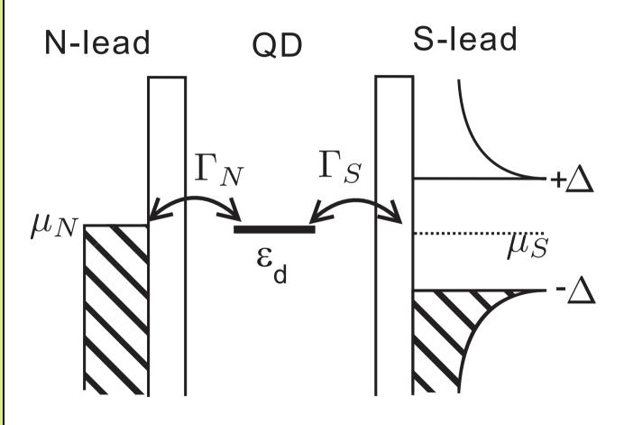
Hybridization of the QD to superconducting lead
