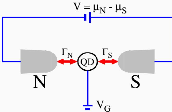
This is a particular realization of the single-electron-transistor.
