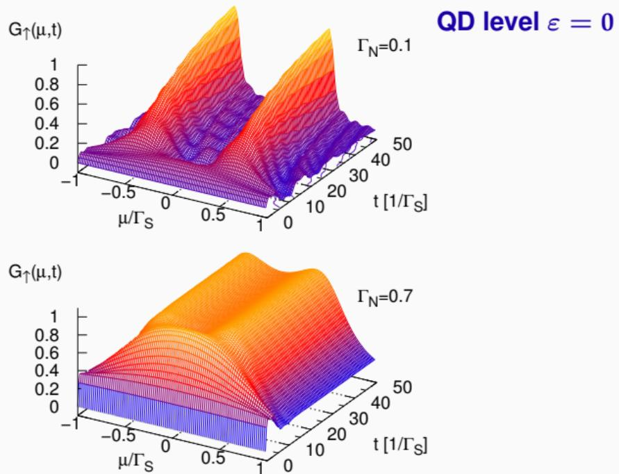
**Subgap tunneling conductance  $G_{\sigma} = \frac{\partial I_{\sigma}}{\partial t}$  vs time (t) and voltage ( $\mu$ )**
