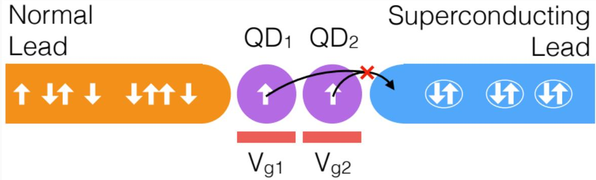
**Problem:** initial triplet configuration does not allow for development of the superconducting proximity effect
