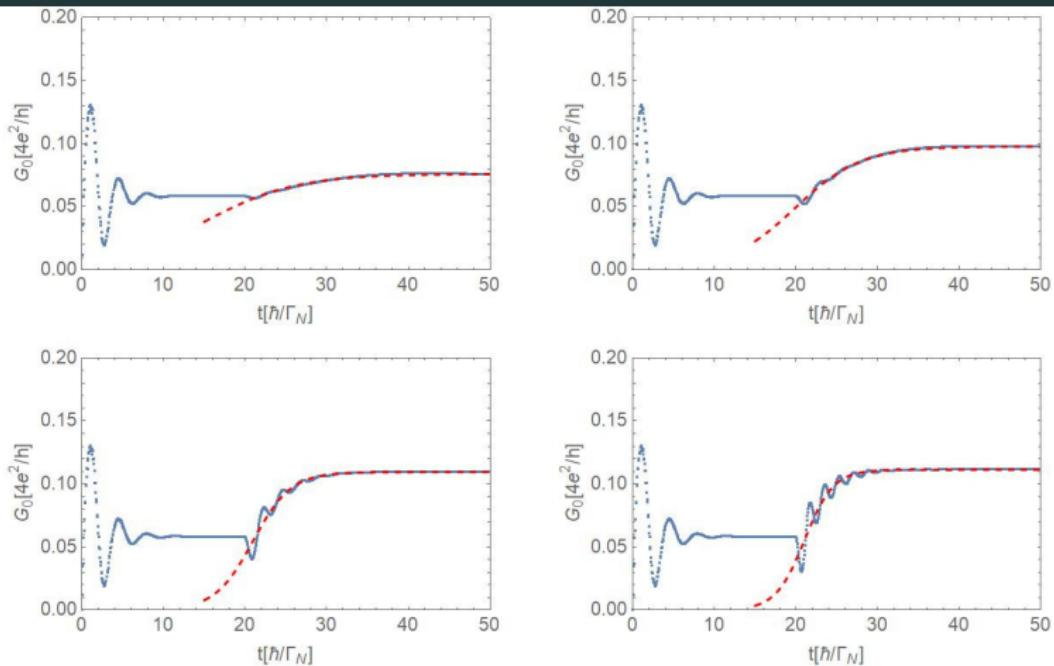
The zero-bias differential conductivity obtained for  $\Gamma_S = 3\Gamma_N$  and  $\epsilon_d = \Gamma_N$ , assuming:  $t_m = 0.25$  (upper left),  $0.5$  (upper right),  $1$  (lower left),  $1.5$  (lower right)  $\Gamma_N$ . QD is abruptly connected to Majorana mode at time  $t = 20\hbar/\Gamma_N$ . Typical values of the Majorana leakage time  $\tau = 2 - 20$  nanoseconds.
