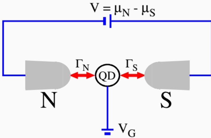
This is particular version of single-electron-transistor (SET) which operates on the Andreev (electron-to-hole) scattering mechanism.
